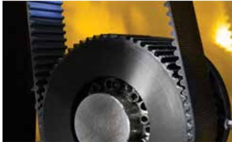
**RELIABLE COMPONENTS** The poly-synchronous belt drum drive helps reduce maintenance and offers adjustable shafts.
