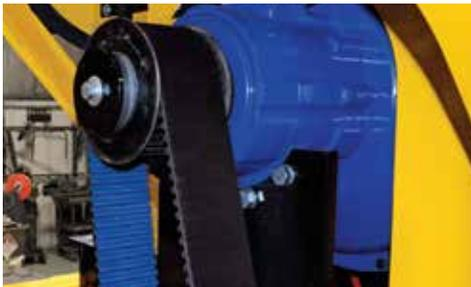
**EXTENDED CLUTCH LIFE.** Engine power is transferred through the hydraulically actuated PT Tech clutch. To help extend clutch life, control software prevents the operator from engaging or disengaging the drum drive at full engine rpm.
