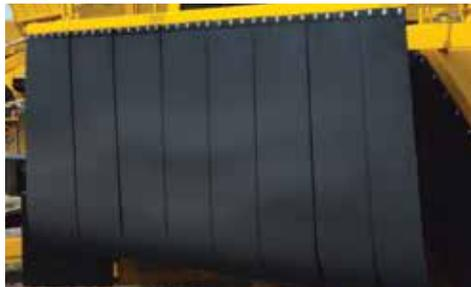
**CONTAINMENT CURTAINS.** Rubber containment curtains draped over the front and back help keep material in the windrow, reducing the quantity and distance of thrown objects.
