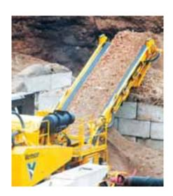
Wide loadout conveyor At 14 to 18' (4.3 to 5.5 m) discharge height for the HG8000, 14.5' (4.4 m) for the HG8000TX, the 66" (168 cm) wide loadout conveyors are the widest around. This allows for greater volume of processing with less chance of spillage or plugging.
