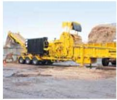
SmartGrind Three preset grinding settings: aggressive, general, and regrind reduce operator training time and result in more consistent end product. A fourth setting can be customized for specific product needs.
