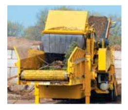
Dual planetary feed roller drive For added torque and greater processing power, the large feed roller features dual planetary drive motors.
