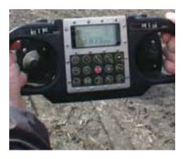
Remote control In addition to most machine functions, the discharge height is adjustable via remote control (trailer unit only), a feature unique to the industry that helps keep operators productive and the machine working efficiently.
