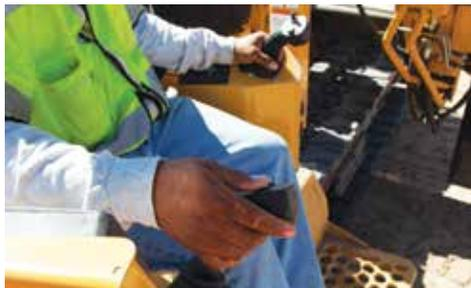
**TAKE CONTROL.** Conveniently placed dual joystick controls allow the operator to control machine functions including engagement of the hammer, pile placement and ground drive.
