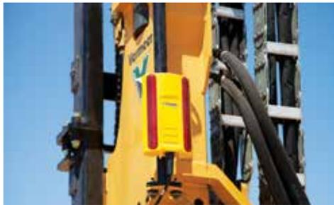
**IMPROVE YOUR ACCURACY.** An optional laser receiver integrated into the control system and a GPS-ready design (capable of accepting a number of different systems) can help improve productivity.
