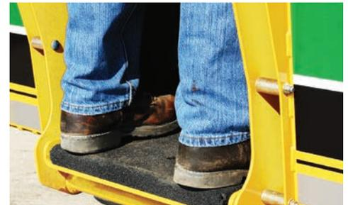
**A DEDICATED SPRING-CUSHIONED PLATFORM** keeps the operator out of the mud. The integrated operator presence system suspends ground drive and powered boom/bucket motion when the operator steps off the platform.
