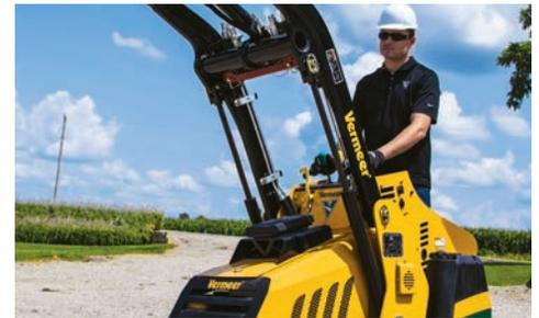
**ISO-RATED OPERATING CAPACITY** for the S725tx is 750 lbs (340.2 kg). With a rated tipping load of 2145 lbs (973 kg), this small footprint machine positions itself as an exceptional mini skid steer. Additionally, the S725tx leads the industry with a lift height (to hinge pin) of 84.5" (214.6 cm).
