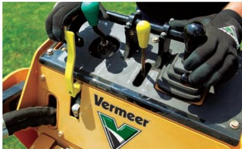
**EFFICIENCY AND PRODUCTIVITY ARE NOW MADE EASY** with a single pilot-operated ground drive joystick, which allows for a smooth range of motion. Additionally, a conveniently placed auxiliary lever by the loader arm controls, allows operators to multitask.
