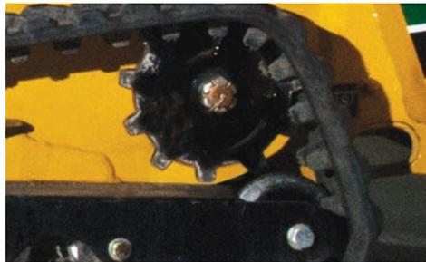
**LOWER YOUR COST OF OPERATION** with a high mounted track sprocket. The higher mounting reduces premature wear and tear in rocky soil conditions, while the ADI cast sprocket is heat-treated for longer life.
